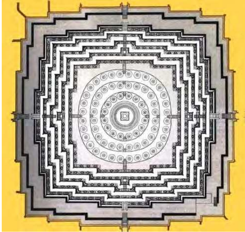
Image 6.3 Plan of Candi Borobudur in Central Java. There are four terraces with relief panels on the lower square platform surmounted by three circular terraces with a bell-shaped stupa at the very crown.
