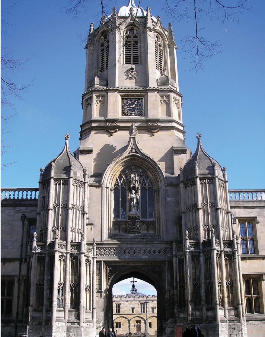
Wren's Gothic Tom Tower, the gatehouse to Christ Church College, Oxford, decorated with an octagonal lantern and pointed ogee arches.
